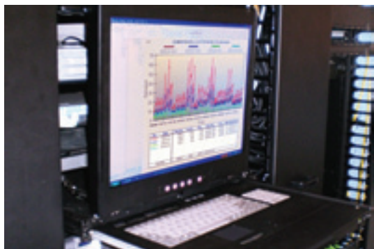
Figure 3: Energy intelligence software allows generation of graphs and profiles of kWh and kW for demand analysis and usage reduction. Converted meter data is presented in both historical and real-time slices for trending and reporting.
