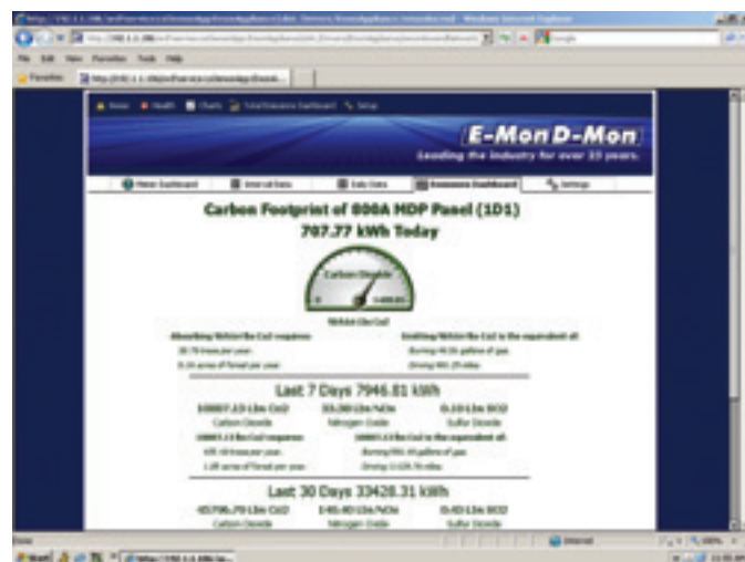
Figure 4. Carbon footprint dashboard of an 800A main distribution panel. The meter data provided by an E-Mon D-Mon Class 3000 submeter is converted by energy intelligence software into real-time and historical kWh statistics, along with generated CO 2 , NO x , SO 2 and other measurements and calculations.
