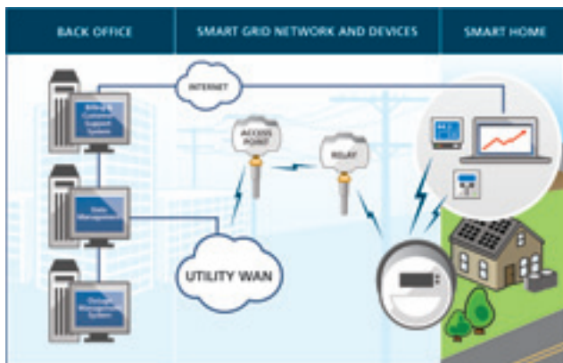
Diagram depicts 2-way communication between the Home Area Network (HAN) and the Wide Area Network (WAN). Electricity usage data is collected at the meter and then distributed to in-home devices within the HAN. At the same time the data is sent out via access points to OG&E's back office via the WAN. That information is then routed back to the consumer via the internet and viewed using myOGEpower.com .
