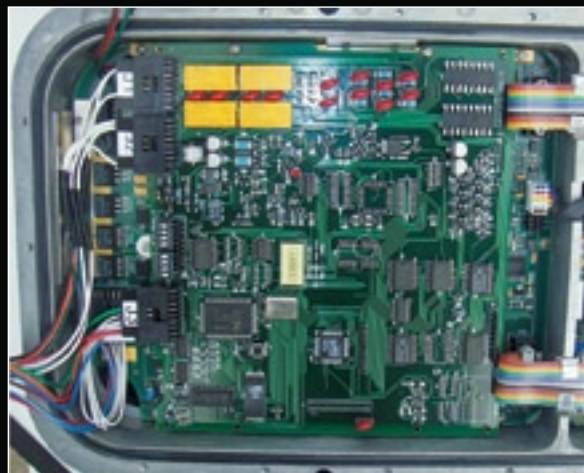
Figure 3: Special interface module installed inside remote satellite terminal
