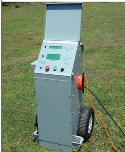
VLF Cable Testing
